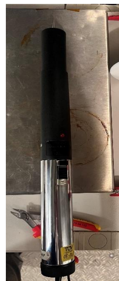
2 High voltage generator with corona charging tip
