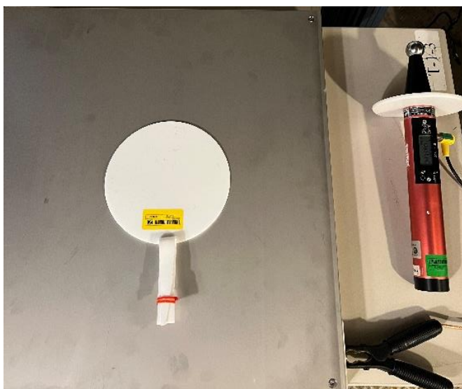
1 Metal plate grounded and reference disc made of PTFE
